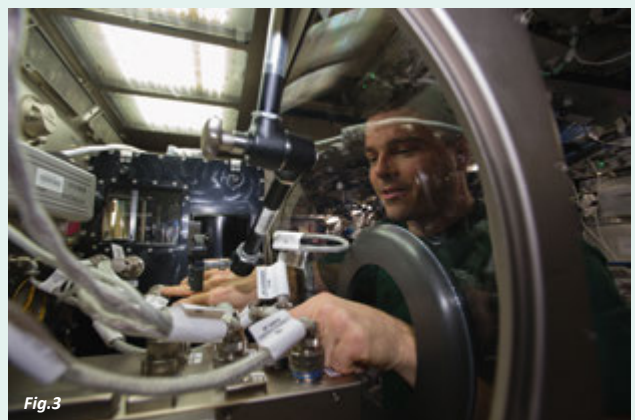
Fig. 3: NASA astronaut Reid Wiseman, Expedition 40 flight engineer, installs Capillary Channel Flow (CCF) experiment hardware in the Microgravity Science Glovebox (MSG) located in the Destiny laboratory of the International Space Station. CCF is a versatile experiment for studying a critical variety of inertial-capillary dominated flows key to spacecraft systems that cannot be studied on the ground. © NASA
