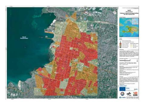
Fig. 1: Cartography of presumed damaged buildings made by SERTIT from satellite imagery © SERTIT
