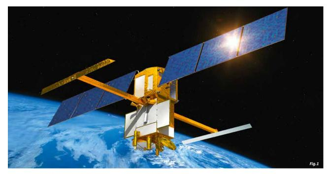
Satellites have already revolutionised oceanography, and tomorrow they will do the same for hydrology. The French-U.S. SWOT mission (Surface Water and Ocean Topography) will be at the forefront, carrying a wide-swath Ka-band radar interferometer dubbed KARIN that marks a break with today's technologies. Four agencies are joining forces to develop the SWOT project: NASA, CNES, CSA, UKSA.
